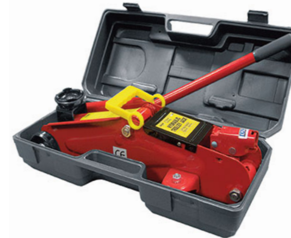
2 TONNE TROLLEY JACK (2000KG) Fitted with swivel castors & easy grab yellow handle to enable easy positioning. Large 360° lifting saddle with lifting range of 135mm - 330mm Extension handle for easy to use operation. SW2TJBM 5026637 610875
