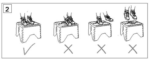
WHEN STEPPING ONTO THE UNIT, PLACE BOTH FEET AND EVENLY DISTRIBUTE WEIGHT ON THE TOP SURFACE. DO NOT JUMP, HOP, OR SHIFT WEIGHT WHILST ON THE PRODUCT.
