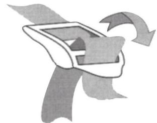
**CAUTION!** Do not pull the straps to the point where the buckle may break. Once all buckles have been secured, check the Cargo Carrier is secure by moving it forward and back and side to side. If cargo carrier can be easily moved continue to tighten the straps until movement has minimized.
