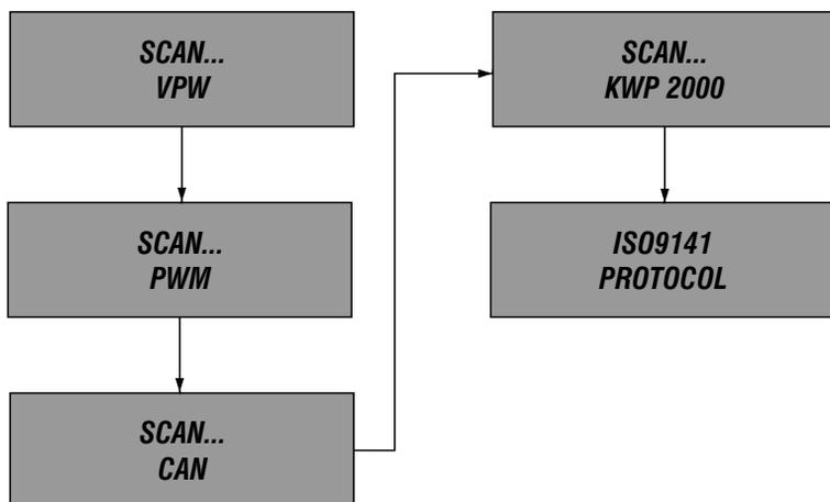
**If a "LINK ERROR!" message shows up, turn the ignition off for about 10 seconds, check if the Scan Tool's OBDII connector is securely connected to the vehicle's DLC, and then turn the ignition back to on. Repeat the procedure from step 5. If the "LINK ERROR" message does not go away, then there may be problems stopping the Scan Tool communicating with the vehicle.**
