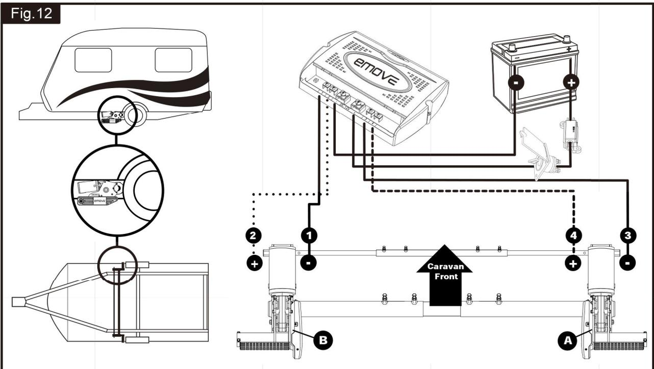
**Parts Identification & Fitting Diagrams**
