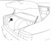
It may be necessary to remove the back panels to mount the control box in a safe place, away from rain, heat or humidity.
