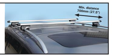
When both roof bars are connected correctly, secure them by locking with the security keys.
