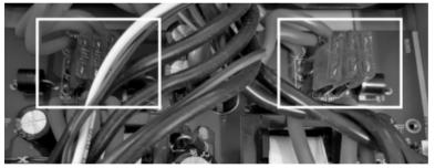
If the unit stops working, and you see a red LED light and/or you hear an audible beeping. Then you will need to check to see if any of the fuses are working, and replace any blown fuses if necessary.
