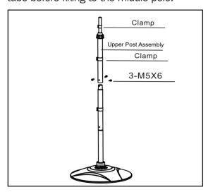
2. Screw 3 x M5, 6mm screws into end of the middle tube and attach the cord support clamp to the middle tube before fixing to the base pole.
