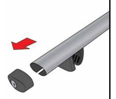
■ When the mounting bracket is mounted on the roof rail, tighten with the allen key until the bracket is tight to the roof rail.
