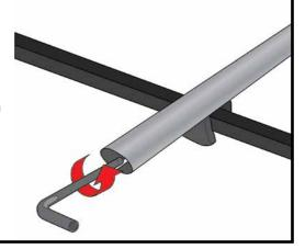
■ Ensure that there is a minimum distance of 700mm (27.5") between the roof bars when mounted on the roof rails.
