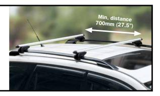
When both roof bars are connected correctly, secure them by locking with the security keys.
