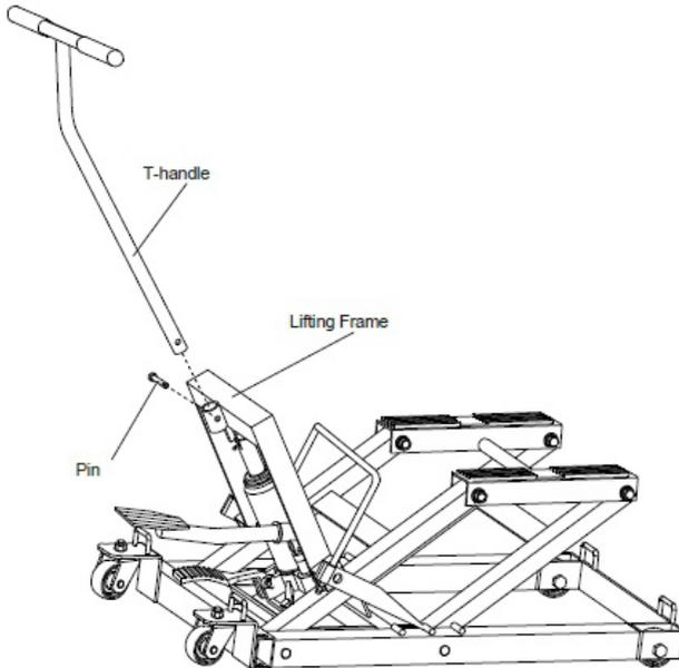
7. The assembly is now complete. Before using the motorcycle jack, ensure the jack can move, lift and lower freely.
