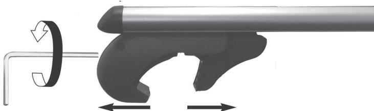
3. Mount the roof bars to your vehicle's roof rails, and use the Allan key to securely tighten the mounting bracket onto the roof bars.
