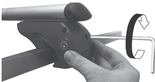
**PLEASE NOTE:** When installing the roof bars, please ensure the mounting bracket is securely connected to the roof rails, as shown below (A). If roof bars are incorrectly mounted (as shown in B & C, this will risk destabilising the load, causing danger to other road users).
