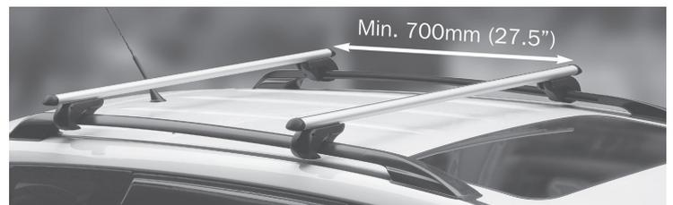
5. Once both roof bars have been mounted and correctly positioned, secure them with the security keys to cover the Allan key access with the red guard.
