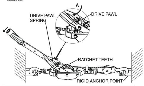
4 Ton pulling capacity is static pulling power. Please consider coefficient of friction when using for heavy loads which will impact upon the overall capacity. The same coefficient of friction will also apply to the maximum lifting capacity of 3 Ton.
