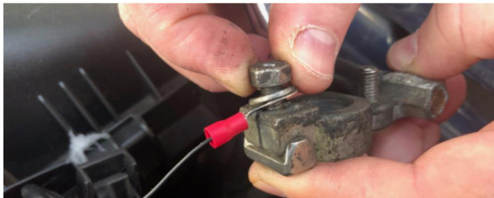
6. Once the connection to the vehicle's battery has been secured, connect the tracker to the other end (USB-end) of the cable.
